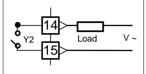
NO contact, capacity 3A/250Vac Load for resistive loads (transition 2 x 10<sup>5</sup> min. at 3A/250Vac)
