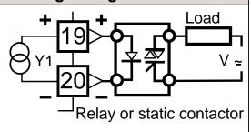
Output 0/15Vdc (20mA max.) galvanically isolated
