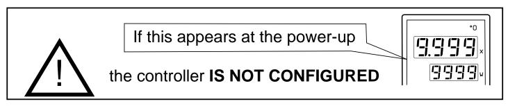
In order to configure the controller, follow the configuration procedure reported in the enclosed leaflet
