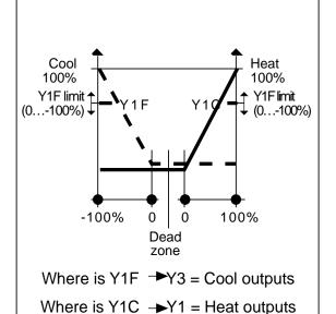
Only for models with option Y3 is possible to have a double action regulation (for instance Heat - Cool). Output Y3 with index H=9, is available as cool output.
