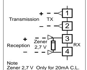
Interface 20mA C.L. passive and galvanically isolated
