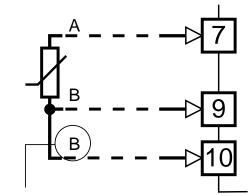
for 3-wire connection only Line: max. 20  $\Omega$  per wire
